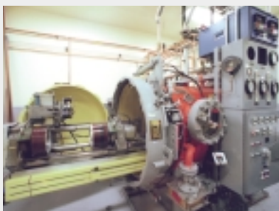
The pressurized inert-gas metal arc welder is used for welding pits.
