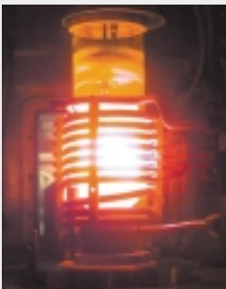
An induction furnace melts plutonium, which is then cast into pits.
