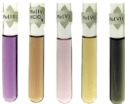
Each plutonium oxidation state has a characteristic color in solution.
